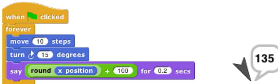
The `round` block rounds 35.3905... to 35, and the `+` block adds 100 to that. (By the way, the `round` block is in the Operators palette, just like `+`, but in this script it's a lighter color with black lettering because `Snap!` alternates light and dark versions of the palette colors when a block is nested inside another block from the same palette:
